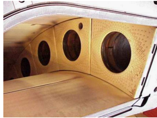
Fig. 23 View into the annular premix combustor of the GT26 (burners and igniter removed)
