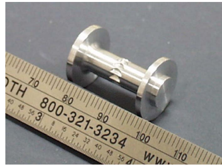
Fig. 5 The rotor hardware with mesoscale turbine
