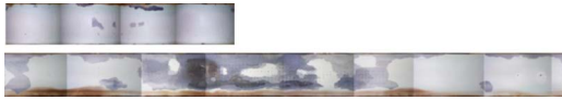
Fig. 14 Digital photographs of (a) HiNi/BN/SiC-Si (MI) inner liner and (b) HiNi/PyC/E-SiC (CVI) outer liner after 7238 h field test (MM-1) [5,18]
