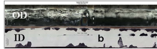
Fig. 16 Digital photographs of (a) TyZM/BN/SiC-Si (MI) inner liner and [23], (b) HiNi/PyC/SiC (CVI) outer liner after 15,144 h field test (MM-2); ID/OD: inner/outer diameter
