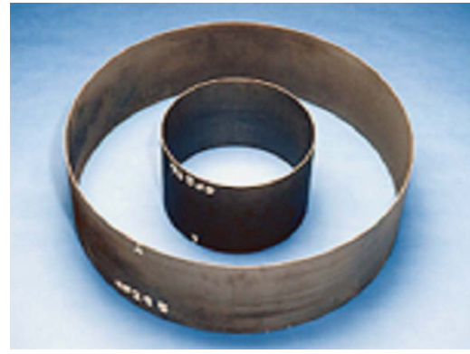
Fig. 5 CG Ni/PyC/E-SiC (CVI) liners before 100 h test
