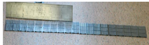
Fig. 6 A section of the hardware for compliant bump foil assembly
