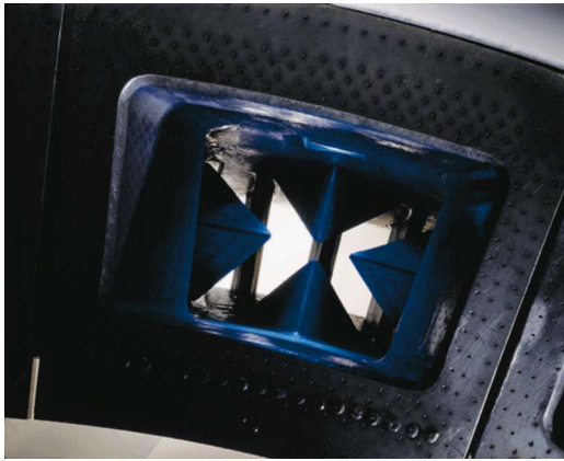
Fig. 17 View from downstream into the SEV burner (fuel lance removed)
